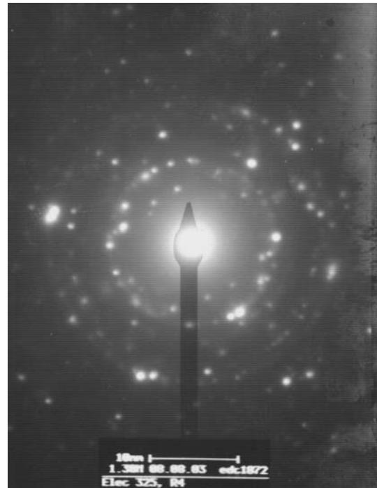
Fig. 9 Electron diffraction pattern of -44\ \mu\text{m} particles, the rings correspond to iron carbides
